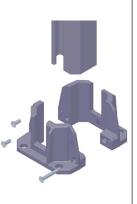
**TIGHTEN** the two halves of the post support against the sides of the post by tightening the 3 installation screws.
