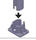
**A13. SCREW** the pressure screws onto the posts using a No.4 Allen key until the assembly no longer moves (hand tightening).
